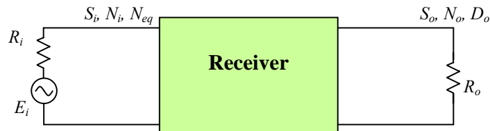
Figure 9.8 The basic parameters in the sensitivity testing for a receiver
