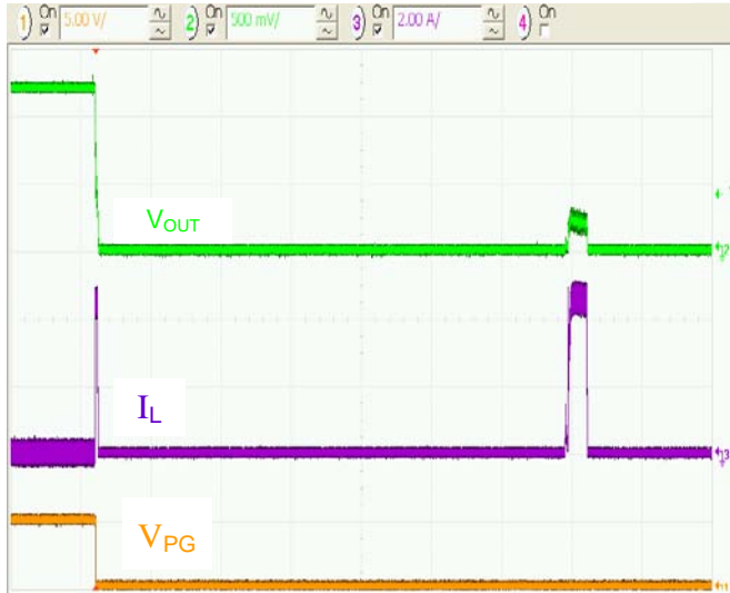
Figure 19. VOUT to GND Short Circuit, 200 \mu\text{s}/\text{div} .
