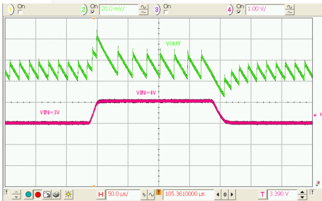
Figure 23. Line Transient, 3-4 V_{IN} , 1.2 V_{OUT} , 10 \mu\text{s} Edge, 50 \Omega Load
