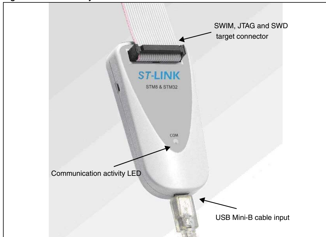
Figure 3. ST-LINK layout
