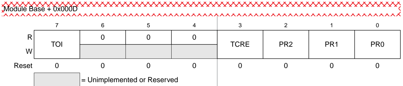
Figure 14-19. Timer System Control Register 2 (TSCR2)
