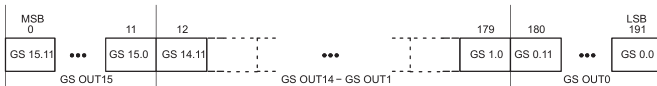
Figure 21. Grayscale Data Packet Format
