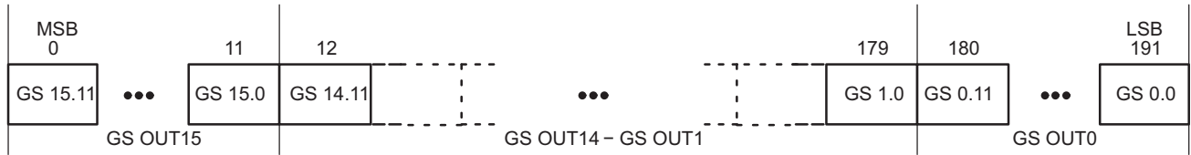
Figure 11. Grayscale Data Packet Format
