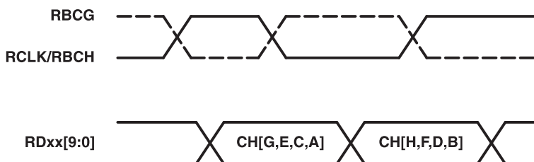
Figure 6. Multiplexed Channel Receive Timing
