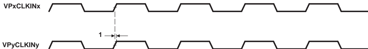
Figure 5-61. Video Port Dual-Display Sync Timing
