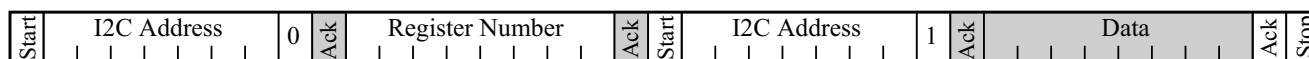
Figure 31. Format of a Register Read. Shaded Regions Denote Bus Control by TPS2358/9
