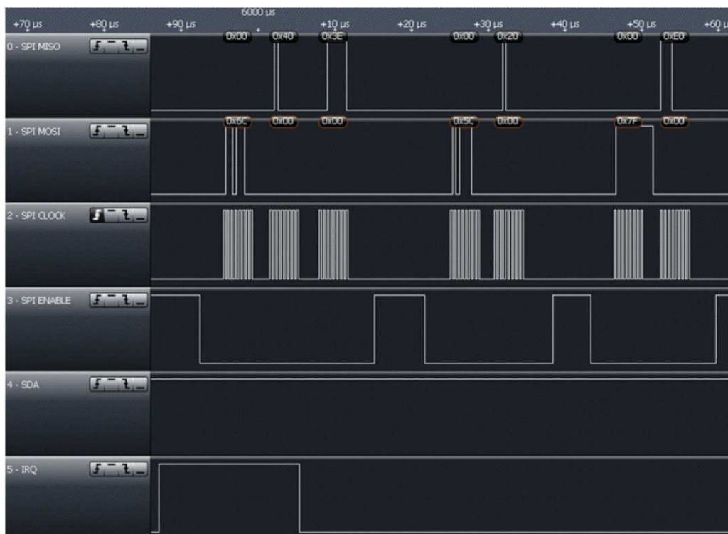
Figure 6-24. IRQ With One Byte in FIFO
