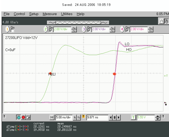
Figure 31. V_{LO} and V_{HO} Rising Edge Delay Matching
