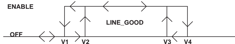
Figure 2. Line UVLO and OVLO Operation
